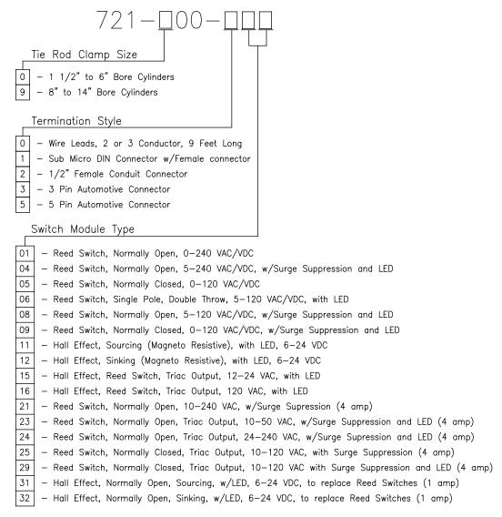
**Note:** When ordering a pneumatic cylinder for use with tie rod mount limit switches, in addition to the cylinder part number, specify "with magnetic piston for reed switch" and reference the reed switch P/N, or "with magnetic piston for hall effect switch" and reference the hall effect switch P/N. Switch not included in cylinder pricing. Order switch separately.
