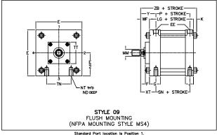
NOTE: THE 14" BORE USES FOUR (4) TIE RODS. BORE SIZES 16"-18"-20" USE EIGHT (8) TIE RODS. (SEE ILLUSTRATIONS ON P.29)
