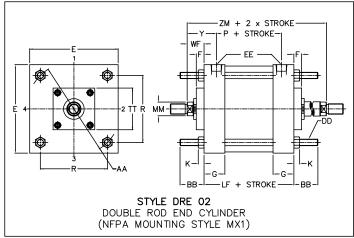
Standard Port location is Position 1. Standard Cushion location Position 2. Standard Port location is Position 1. Standard Cushion location Position 2.
