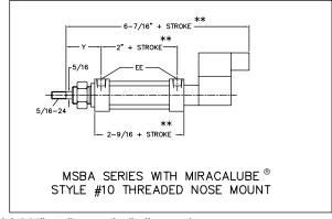
\*\*For spring return cylinder, add 3/4" to "+ stroke" dimension
