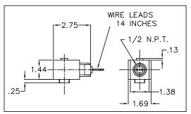
The special electrical coil shown at the left is available at extra charge. This water-tight and explosion proof enclosure is for indoor or outdoor use in NEMA groups 4, 6, 7C, 7D, 9E, 9F 9G and 12.
