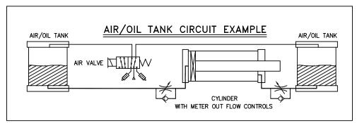
**Note:** Sample circuits are for concept illustration purposes only. Additional safety devices, controls and lockouts are required for safe operation.
