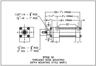
Standard Port location is Position 1 Standard Cushion location Position 2 NOTE: For 1-1/2", 2", 2-1/2" cylinder only with 5/8" and 1" rod sizes only
