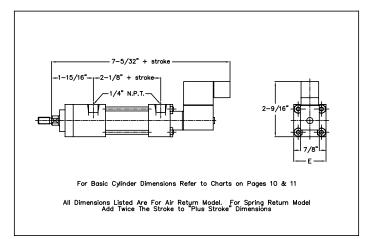
The JHDA 01 series air motor combines the rugged 1" dia. bore JHD 01 heavy duty air cylinder (pp.12-13) with an electric solenoid valve to create a cylinder and valve designed as a unit. One electrical connection and a single air supply line to the valve-in-head end of the cylinder simplifies installation. (For an air return model, a constant pressure air line must be connected to the rod end port of the cylinder.)
