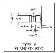
Note: "V" dimension varies per bore size. See data in mounting dimension tables of the respective cylinder mounts.
