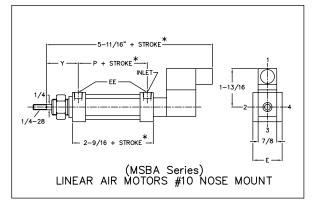
\*For spring return cylinder, add twice stroke to "+ stroke" dimension
