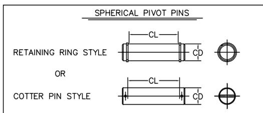
Note: Pivot pin is not supplied with any spherical rod end or cap end mounting accessory. It must be ordered as separate item if required.
